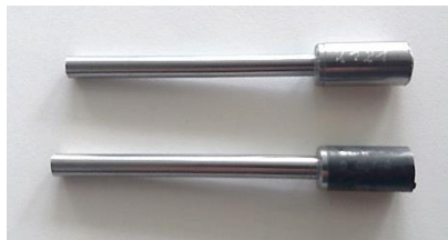
Figure 16: Example of steel samples used for hardening (at right end: identification code)
