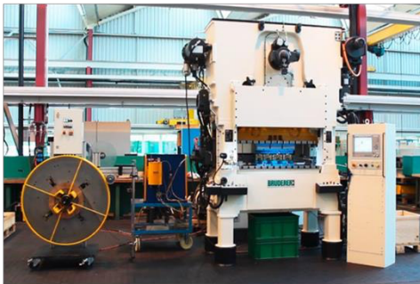
Figure 8: Lab scale cutting test at Fraunhofer IWU with “Dreieckgeometrie”, stainless steel 1.4301
