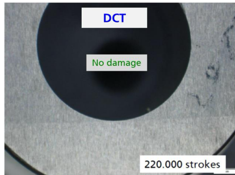
Figure 70: Industrial HSIC cutting test of solid copper. Tool wear after 220.000 strokes (CHT and DCT)
