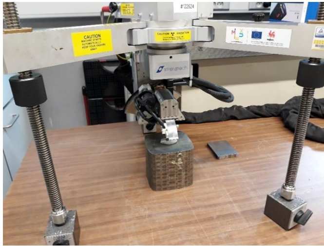
Figure 25: Set-up of the mobile residual stress measuring apparatus Stresstech
