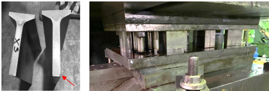
Figure 68: Side cutters from the industrial cutting test at Haemers NV (left: XS=DCT), right punching dies with side cutters
