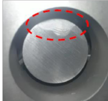
Figure 49: High speed impact cutting, punch after 35 strokes
