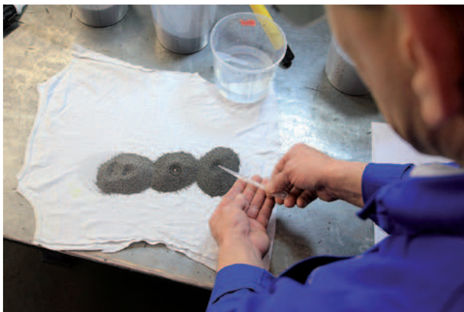
PantaTec_Water penetration test
