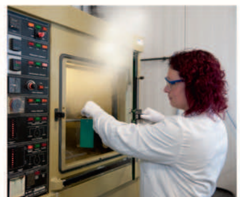
Test chamber neutral salt spray test
