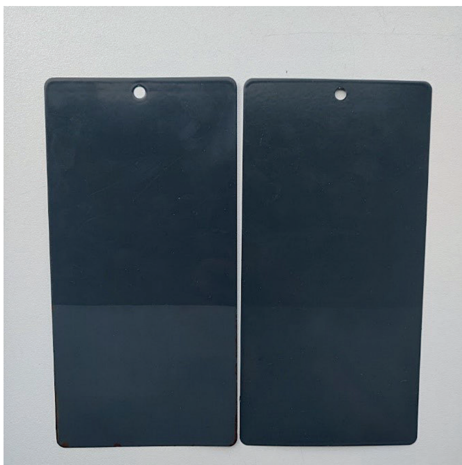
▲ Figuur 1 Verkleuring Qualicoat waterspot test QUALICOAT Water Sport test: - Links: Standaard polyester RAL 7016 (DE=3.40) - Rechts: Qualicoat polyester PE50 RAL 7016 (DE=0.60)
