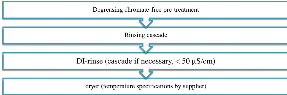
Beside the chromate-free corrosion protection process (product name) the used process variant is specified in the certificate of approval. As the approval test only includes the corrosion protection characteristics of the chromate-free pre-treatment product, the cleaning product will not be specified.
