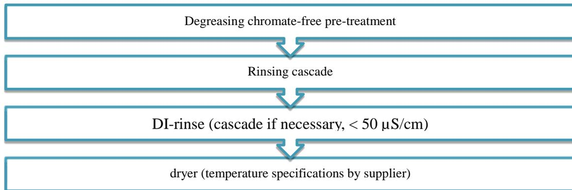
4.6.2 Strip galvanising or hot-dip galvanising according to ISO 1461:
